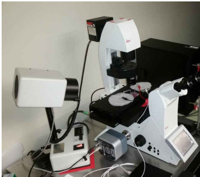
Figure 4. Experimental setup for imaging monolayers during electrotaxis
